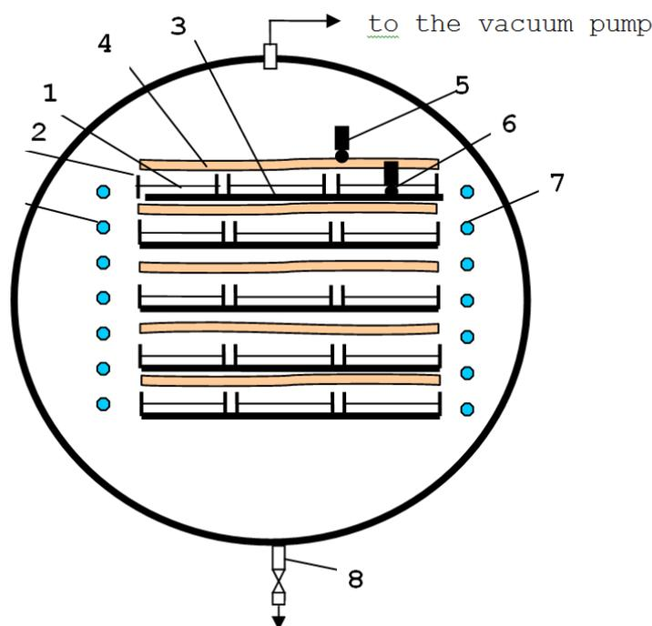
**Figure: The diagram of vacuum drying plant with infrared transmitters VDSU-2M**
